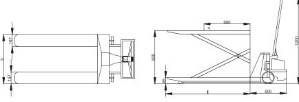
All parts are made of stainless including hydraulic pump fork frame , handle , push rod, Bearing pin and bolt , etc. for use in meat and other food industry, dairy canning and all area where corrosive acids and sailine are used.
